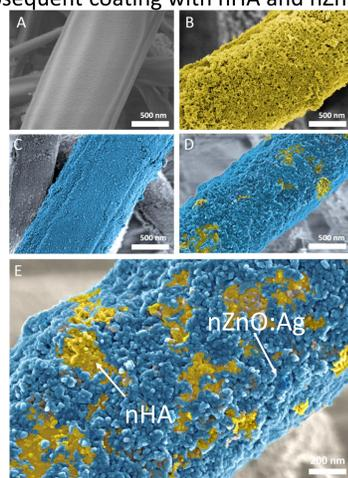
Fig.3 Colored SEM image of: A) non-coated PDLLA/PLGA fiber, B) PDLLA/PLGA/nHA, C) PDLLA/PLGA/nZnO:Ag, D) PDLLA/PLGA/nHA/nZnO:Ag after coating and E) PDLLA/PLGA/nHA/nZnO:Ag after 24h immersion in PBS medium at 37 °C.
