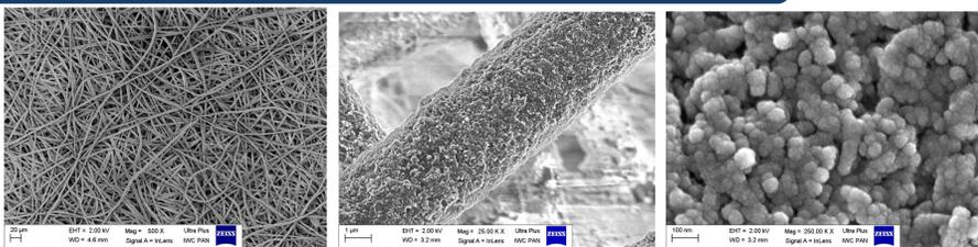
Fig.3 Colored SEM image of: A) non-coated PDLLA/PLGA fiber, B) PDLLA/PLGA/nHA, C) PDLLA/PLGA/nZnO:Ag, D) PDLLA/PLGA/nHA/nZnO:Ag after coating and E) PDLLA/PLGA/nHA/nZnO:Ag after 24h immersion in PBS medium at 37 °C.
