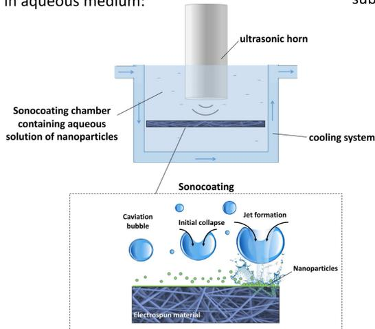
Fig.2 The scheme of sonocoating process. Source: Higuchi J, et al. Polymer Membranes Sonocoated and Electrospayed with Nano-Hydroxyapatite for Periodontal Tissues Regeneration, Nanomaterials 2019, 9, 1625; doi:10.3390/nano9111625.
