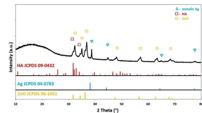
Fig.5 X-ray diffraction patterns of the PDLLA/PLGA/nHA/nZnO:Ag sample correlated with JCPDS data for HA, Ag, and ZnO.
